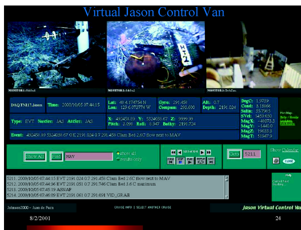
Figure 7. The Virtual Jason Control Van is a web-based application that takes real-time snapshots of information occurring inside the control van during vehicle operations and makes this information immediately available for shipboard scientists and for collaboration and post-cruise analysis on shore. Features include monitoring real-time operations, searching for events, dates, etc. Figure courtesy of Steven Lerner (WHOI).
